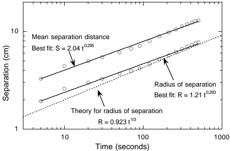
Figure 14. Observed radius of separation and mean separation of three flame balls in Test #1 as a function of time, and comparison to theoretical predictions<sup>16</sup>.
