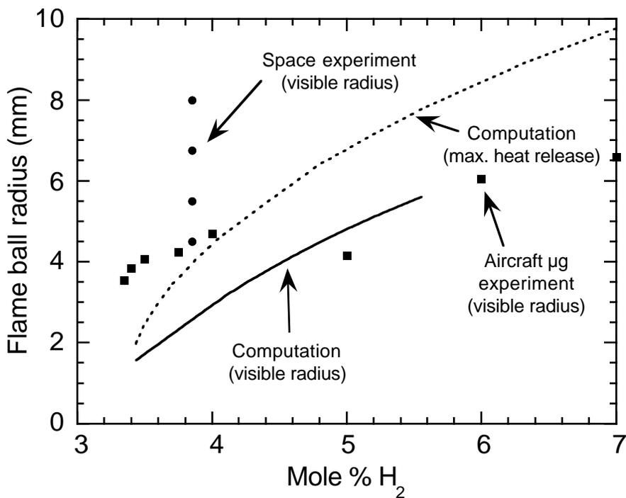
Figure 10. Predicted<sup>13</sup> visible flame ball radii in  $H_2$ -air mixtures (solid curve) along with measured flame ball radii from aircraft  $\mu g$  experiments<sup>7</sup> (squares) and preliminary measured radii for Test #2 (circles). Also shown are predicted<sup>13</sup> flame ball radii based on radial location of maximum heat release. The GRI chemical mechanism<sup>17</sup> is used in the predictions shown.
