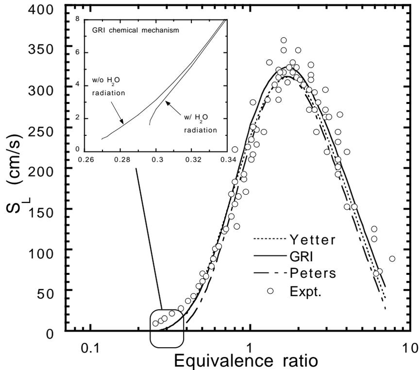
Figure 4. Predicted<sup>13</sup> steady burning velocities ( $S_L$ ) of H<sub>2</sub>-air mixtures using the GRI<sup>17</sup>, Peters<sup>18</sup> and Yetter<sup>19</sup> chemical models. A compilation<sup>20</sup> of experimental results from several sources is also shown.
