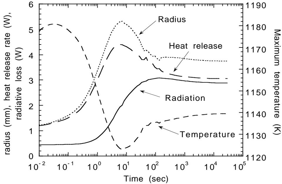
Figure 5. Predicted nonsteady evolution of a flame ball in a 4.02% H<sub>2</sub>-air mixture<sup>11</sup>. “Radius” refers to radial location of maximum volumetric heat release rate; “heat release rate” and “radiative loss” refer to total values (integrated over all radii).
