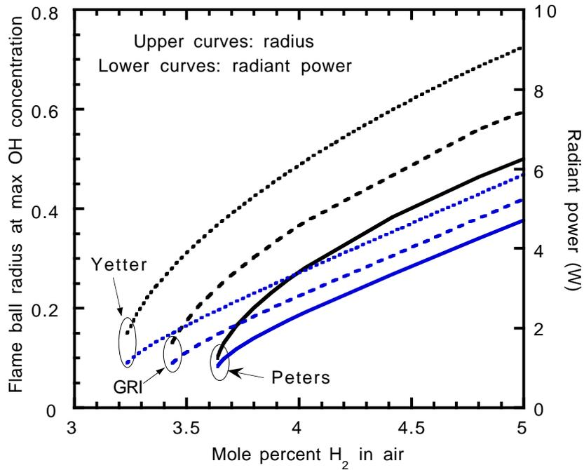
Figure 3. Predicted<sup>13</sup> steady flame ball radii and radiant emission in H<sub>2</sub>-air mixtures using the GRI<sup>17</sup>, Peters<sup>18</sup> and Yetter<sup>19</sup> chemical models.
