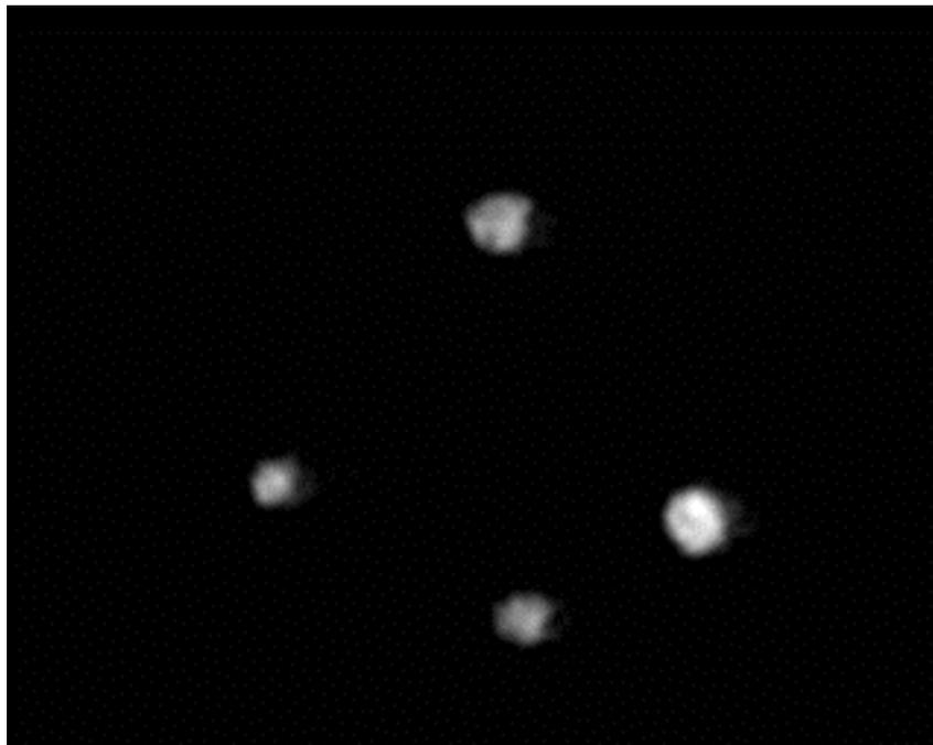
Figure 9. Image of flame balls obtained in 3.85%  $H_2$  / 96.15% air mixture, taken 25 s after ignition. Field of view is 112 mm x 150 mm.
