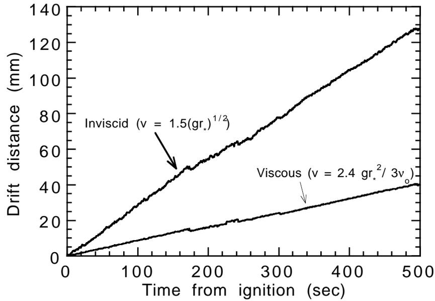
Figure 13. Flame ball drift distances predicted by the inviscid (Eq. (2)) and viscous (Eq. (4)) bubble rise relations for the conditions of Test #1, using acceleration data from the MMA/ASTRE system.
