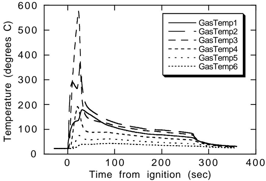
Figure 11. Measured gas temperatures for Test #2. Thermocouple locations corresponding to GasTemp1 through GasTemp6 are 30, 50, 70, 90, 110 and 130 mm from spark gap, respectively.
