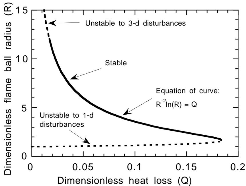
Figure 2. Theoretical prediction<sup>8</sup> of the effect of heat loss on flame ball radius and stability properties with single-step Arrhenius chemistry, constant thermodynamic and transport properties and volumetric heat loss from the interior of the ball. The dimensionless radius is the ratio of  $r_*$  to the value of  $r_*$  for an adiabatic flame ball in the same mixture. The curve is valid for any Lewis number, but the stability properties shown apply to  $Le < 1$  only.
