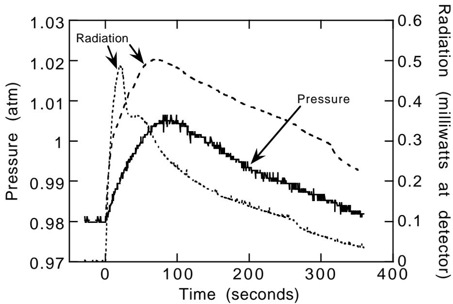
Figure 12. Measured chamber pressure and radiant emissions for Test #2.
